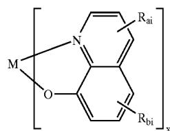
[0046] M is a metal selected from the group consisting of Ca, Sr, Ba, Ti, Zr, Hf, V, Nb, Mo, W, Mn, Tc, Re, Fe, Ru, Os, Ni, Pd, Pt, Zn, Cd, Hg, Ge, Sn, and Pd. Zr and Hf are preferred metals. x is the number of bidentate ligands that may be attached to the metal. For example, if M is Zr or Hf, then x is 4. Rai and Rbi each represent no substitution, mono-, di-, or tri- substitution. If there are substituents, the
