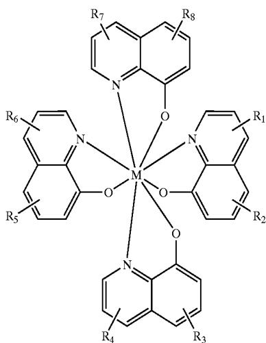
[0050] M is a metal selected from the group consisting of Ti, Zr, Hf, Nb, Re, Sn and Ge. Preferred metals include Zr
